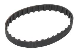
SureMotion timing belt, 3/8in L pitch, 1/2in wide, 33 tooth, 12.4in pitch length (circumference), neoprene, fiberglass reinforced.
