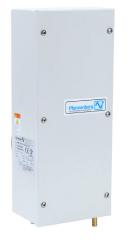
Pfannenberg air-to-water heat exchanger, 3241 BTU/H, 115 VAC operating voltage, 60 Hz, 0.69A running current, side mount, galvanized steel, RAL 7035 light gray, powder coat finish. For use with NEMA/UL Type 3R & 4 enclosures.
