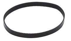
SureMotion timing belt, 0.08in MXL pitch, 1/4in wide, 122 tooth, 9.8in pitch length (circumference), polyurethane, polyester reinforced. Package of 3.
