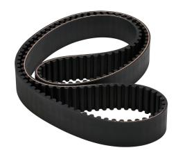
SureMotion timing belt, 8mm 8M pitch, 30mm wide, 153 tooth, 1224mm pitch length (circumference), neoprene, fiberglass reinforced.
