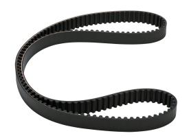
SureMotion timing belt, 8mm 8M pitch, 20mm wide, 153 tooth, 1224mm pitch length (circumference), neoprene, fiberglass reinforced.
