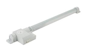
Stego Varioline LED enclosure light, 120 VAC operating voltage, no switch, 27.3in length, 1730 Lm, integral receptacle, magnet mount, 3-pole plug with snap lock, 16W, IP20.
