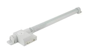
Stego Varioline LED enclosure light, 120 VAC operating voltage, connection for external switch, 27.3in length, 1730 Lm, integral receptacle, magnet mount, 3-pole plug with snap lock, 16W, IP20.
