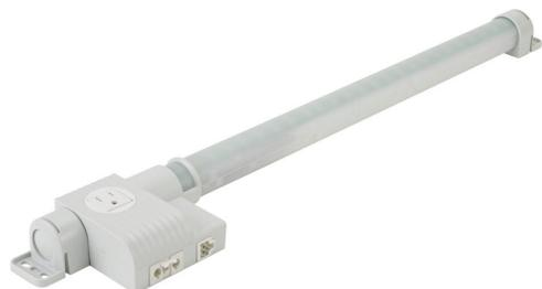
Stego Varioline LED enclosure light, 120 VAC operating voltage, connection for external switch, 27.3in length, 1730 Lm, integral receptacle, screw mount, 3-pole plug with snap lock, 16W, IP20.
