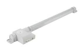
Stego Varioline LED enclosure light, 120 VAC operating voltage, connection for external switch, 27.3in length, 1730 Lm, integral receptacle, screw mount, 3-pole plug with snap lock, 16W, IP20.
