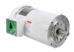
Leeson Washguard White Duck standard efficiency AC induction motor, washdown and inverter rated, 3hp, 3-phase, 208-230/460 VAC, 3600rpm, TEFC, NEMA 145TC frame, rolled steel, C-face mount.
