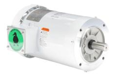
Leeson Washguard White Duck premium efficiency AC induction motor, washdown and inverter rated, 2hp, 3-phase, 208-230/460 VAC, 1800rpm, TEFC, NEMA 145TC frame, rolled steel, C-face mount.
