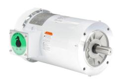
Leeson Washguard White Duck premium efficiency AC induction motor, washdown and inverter rated, 2hp, 3-phase, 208-230/460 VAC, 1800rpm, TEFC, 145TC frame, rolled steel, C-face mount.
