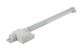
Stego Varioline LED enclosure light, 120 VAC operating voltage, motion sensor switch, 27.3in length, 1730 Lm, integral receptacle, screw mount, 3-pole plug with snap lock, 16W, IP20.
