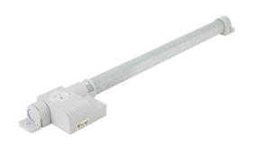
Stego Varioline LED enclosure light, 120 VAC operating voltage, on/off switch, 27.3in length, 1730 Lm, integral receptacle, magnet mount, 3-pole plug with snap lock, 16W, IP20.
