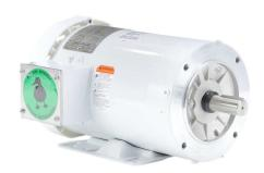
Leeson Washguard White Duck premium efficiency AC induction motor, washdown and inverter rated, 3hp, 3-phase, 230/460 VAC, 3600rpm, TEFC, NEMA 145C frame, rolled steel, C-face/rigid base mount.
