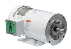
Leeson Washguard White Duck premium efficiency AC induction motor, washdown and inverter rated, 2hp, 3-phase, 230/460 VAC, 1800rpm, TEFC, NEMA 145TC frame, rolled steel, C-face/rigid base mount.
