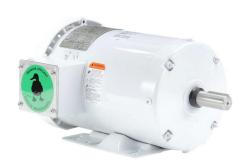
Leeson Washguard White Duck premium efficiency AC induction motor, washdown and inverter rated, 2hp, 3-phase, 208-230/460 VAC, 1800rpm, TEFC, NEMA 145T frame, rolled steel, rigid base mount.
