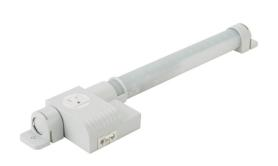
Stego Varioline LED enclosure light, 120 VAC operating voltage, no switch, 19.5in length, 1080 Lm, integral receptacle, magnet mount, 3-pole plug with snap lock, 11W, IP20.
