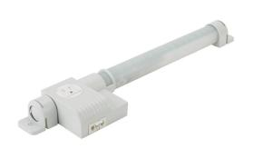
Stego Varioline LED enclosure light, 120 VAC operating voltage, no switch, 19.5in length, 1080 Lm, integral receptacle, magnet mount, 3-pole plug with snap lock, 11W, IP20.
