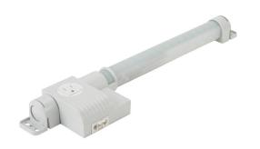
Stego Varioline LED enclosure light, 120 VAC operating voltage, no switch, 19.5in length, 1080 Lm, integral receptacle, screw mount, 3-pole plug with snap lock, 11W, IP20.
