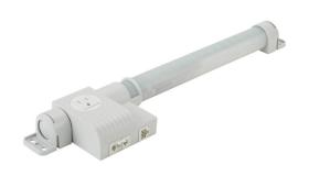
Stego Varioline LED enclosure light, 120 VAC operating voltage, connection for external switch, 19.5in length, 1080 Lm, integral receptacle, screw mount, 3-pole plug with snap lock, 11W, IP20.
