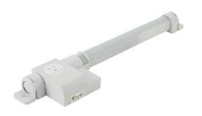
Stego Varioline LED enclosure light, 120 VAC operating voltage, motion sensor switch, 19.5in length, 1080 Lm, integral receptacle, magnet mount, 3-pole plug with snap lock, 11W, IP20.
