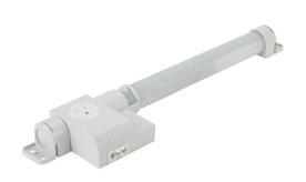
Stego Varioline LED enclosure light, 120 VAC operating voltage, motion sensor switch, 19.5in length, 1080 Lm, integral receptacle, screw mount, 3-pole plug with snap lock, 11W, IP20.
