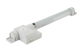
Stego Varioline LED enclosure light, 120 VAC operating voltage, on/off switch, 19.5in length, 1080 Lm, integral receptacle, screw mount, 3-pole plug with snap lock, 11W, IP20.
