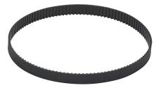
SureMotion timing belt, 0.08in MXL pitch, 1/4in wide, 120 tooth, 9.6in pitch length (circumference), neoprene, fiberglass reinforced. Package of 3.
