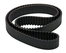
SureMotion timing belt, 8mm 8M pitch, 30mm wide, 150 tooth, 1200mm pitch length (circumference), neoprene, fiberglass reinforced.
