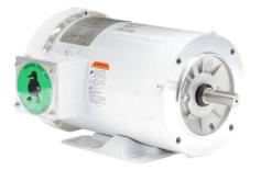
Leeson Washguard White Duck premium efficiency AC induction motor, washdown and inverter rated, 1-1/2hp, 3-phase, 208-230/460 VAC, 1800rpm, TEFC, NEMA 56C frame, rolled steel, C-face/rigid base mount.
