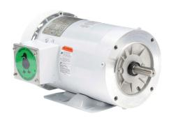
Leeson Washguard White Duck high efficiency AC induction motor, washdown and inverter rated, 1hp, 3-phase, 208-230/460 VAC, 1200rpm, TEFC, NEMA 56HC frame, rolled steel, C-face/rigid base mount.
