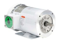
Leeson Washguard White Duck high efficiency AC induction motor, washdown and inverter rated, 1hp, 3-phase, 208-230/460 VAC, 1200rpm, TEFC, 56HC frame, rolled steel, C-face/rigid base mount.
