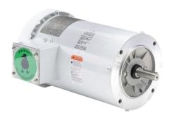
Leeson Washguard White Duck premium efficiency AC induction motor, washdown and inverter rated, 2hp, 3-phase, 208-230/460 VAC, 1800rpm, TEFC, NEMA 56C frame, rolled steel, C-face mount.
