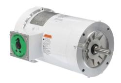
Leeson Washguard White Duck premium efficiency AC induction motor, washdown and inverter rated, 1-1/2hp, 3-phase, 208-230/460 VAC, 1800rpm, TEFC, NEMA 56C frame, rolled steel, C-face mount.
