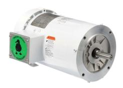
Leeson Washguard White Duck premium efficiency AC induction motor, washdown and inverter rated, 1hp, 3-phase, 208-230/460 VAC, 1800rpm, TEFC, NEMA 56C frame, rolled steel, C-face mount.
