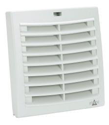
Stego Filter Fan Plus FPO grille, side mount, G3 (coarse) filter mat, NEMA 12,  $4.88 \times 4.88$ in enclosure cutout, RAL 7035 light gray.
