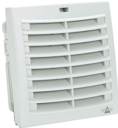
Stego Filter Fan Plus FPI exhaust grille, side mount, with air flaps, NEMA 12, 4.88 x 4.88in enclosure cutout, RAL 7035 light gray.
