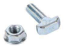
FATH hammer screw, silver, M8-1.25 x 25mm, zinc plated steel, slot size 10. For use with all 45mm and 90mm profile T-slotted rails. Flange nut included. Manufacturer part number: 096HK1030M0825S11.
