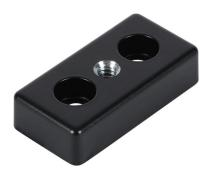
FATH transport/base plate, black, 1 x 2in, 1/4-20 UNC, die-cast zinc, slot size 6. For use with 1 x 2in profile T-slotted rails. Mounting hardware included. Manufacturer part number: 093T25501/406SS01.
