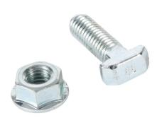
FATH hammer screw, silver, M8-1.25 x 25mm, zinc plated steel, slot size 8. For use with all 40mm and 80mm profile T-slotted rails. Flange nut included. Manufacturer part number: 096HK0830M0825S01.
