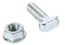
FATH hammer screw, silver, M8-1.25 x 25mm, zinc plated steel, slot size 8. For use with all 40mm and 80mm profile T-slotted rails. Flange nut included. Manufacturer part number: 096HK0830M0825S01.
