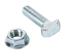
FATH hammer screw, silver, 5/16-18 UNC x 1in, zinc plated steel, slot size 8. For use with all 1.5in and 3in profile T-slotted rails. Flange nut included. Manufacturer part number: 096HK0830U5/16S01.
