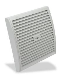
Stego Filter Fan grille, side mount, G3 (coarse) filter mat, NEMA 12, 9.84 x 9.84in enclosure cutout, RAL 7035 light gray.
