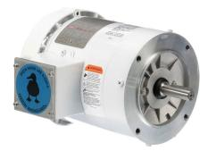
Leeson Washguard White Duck standard efficiency AC induction motor, washdown and inverter rated, 3/4hp, 3-phase, 208-230/460 VAC, 1800rpm, TEFC, 56C frame, rolled steel, C-face mount.
