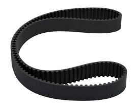
SureMotion timing belt, 8mm 8M pitch, 30mm wide, 145 tooth, 1160mm pitch length (circumference), neoprene, fiberglass reinforced.
