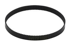
SureMotion timing belt, 0.08in MXL pitch, 1/4in wide, 115 tooth, 9.2in pitch length (circumference), polyurethane, polyester reinforced. Package of 3.
