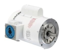
Leeson Washguard White Duck premium efficiency AC induction motor, washdown, 1hp, 1-phase, 115/208-230 VAC, 1800rpm, TEFC, NEMA 56C frame, rolled steel, C-face mount.
