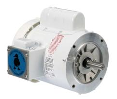
Leeson Washguard White Duck standard efficiency AC induction motor, washdown, 1/2hp, 1-phase, 115/208-230 VAC, 1800rpm, TEFC, NEMA 56C frame, rolled steel, C-face mount.
