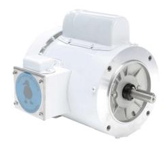
Leeson Washguard White Duck standard efficiency AC induction motor, washdown, 1/3hp, 1-phase, 115/208-230 VAC, 1800rpm, TEFC, NEMA 56C frame, rolled steel, C-face mount.
