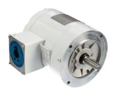
Leeson Washguard White Duck standard efficiency AC induction motor, washdown and high-performance inverter duty, 1/4hp, 3-phase, 208-230/460 VAC, 1800rpm, TENV, NEMA 56C frame, rolled steel, C-face mount.
