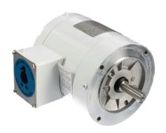
Leeson Washguard White Duck standard efficiency AC induction motor, washdown and high-performance inverter duty, 1/4hp, 3-phase, 208-230/460 VAC, 1800rpm, TENV, 56C frame, rolled steel, C-face mount.
