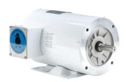
Leeson Washguard White Duck premium efficiency AC induction motor, washdown and high-performance inverter duty, 1-1/2hp, 3-phase, 230/460 VAC, 3600rpm, TENV, NEMA 56HC frame, rolled steel, C-face/rigid base mount.
