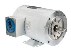
Leeson Washguard White Duck premium efficiency AC induction motor, washdown and high-performance inverter duty, 1hp, 3-phase, 230/460 VAC, 3600rpm, TENV, NEMA 56C frame, rolled steel, C-face/rigid base mount.
