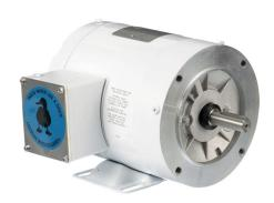
Leeson Washguard White Duck premium efficiency AC induction motor, washdown and high-performance inverter duty, 1/2hp, 3-phase, 230/460 VAC, 1800rpm, TENV, NEMA 56C frame, rolled steel, C-face/rigid base mount.
