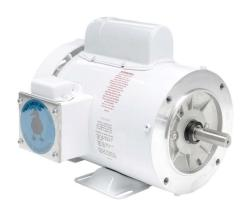
Leeson Washguard White Duck standard efficiency AC induction motor, washdown, 1hp, 1-phase, 115/208-230 VAC, 3600rpm, TEFC, NEMA 56C frame, rolled steel, C-face/rigid base mount.
