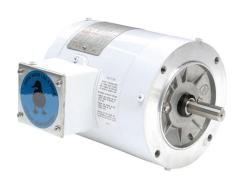
Leeson Washguard White Duck premium efficiency AC induction motor, washdown and high-performance inverter duty, 1/2hp, 3-phase, 208-230/460 VAC, 1800rpm, TENV, NEMA 56C frame, rolled steel, C-face mount.
