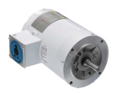
Leeson Washguard White Duck premium efficiency AC induction motor, washdown and high-performance inverter duty, 1hp, 3-phase, 230/460 VAC, 3600rpm, TENV, NEMA 56C frame, rolled steel, C-face mount.
