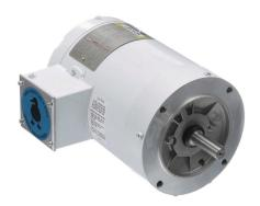
Leeson Washguard White Duck premium efficiency AC induction motor, washdown and high-performance inverter duty, 1hp, 3-phase, 230/460 VAC, 3600rpm, TENV, 56C frame, rolled steel, C-face mount.
