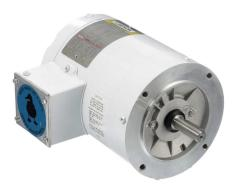
Leeson Washguard White Duck standard efficiency AC induction motor, washdown and high-performance inverter duty, 3/4hp, 3-phase, 208-230/460 VAC, 1800rpm, TENV, NEMA 56C frame, rolled steel, C-face mount.
