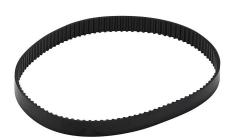
SureMotion timing belt, 0.08in MXL pitch, 1/4in wide, 112 tooth, 9in pitch length (circumference), polyurethane, polyester reinforced. Package of 3.
